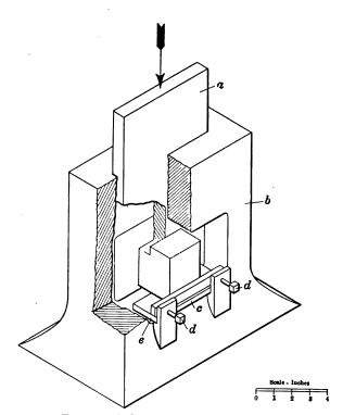
Fig. 8.—Method of making shearing test.
